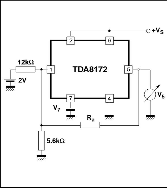
Figure 5. AC test circuit
