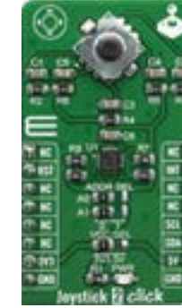
Joystick 2 Click With a SKRHABE01, a 4-direction joystick switch with Center-push Function. MSRP - $15 00 MIKROE-3711
