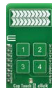
Cap Touch 5 Click Features the CY-8CMBR3106S-LQXI CapSense® Express™ controller. MSRP - $15 00 MIKROE-3786
