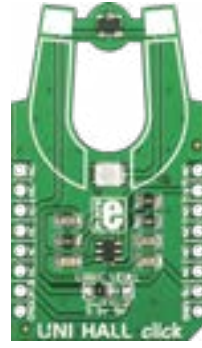
UNI HALL Click With US5881 unipolar Hall-effect switch sensitive to the North Pole magnetic fields. MSRP - $12 00 MIKROE-1647
