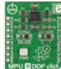
MPU 9DOF Click Carries the MPU-9150 system in package, the world's first 9-axis motion tracking device.
