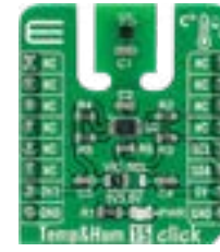
Temp&Hum 15 Click The SHT40, high-accuracy ultra-low-power 16-bit relative humidity and temperature sensor.
