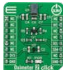
Oximeter 2 Click The ADPD144RI, a PPG optical sensor for photoplethysmography detection of blood oxygenation.
