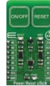
Power/Reset Click It's the QT1011, digital burst mode charge-transfer sensor - detects near proximity or touch. MSRP - $7 00 MIKROE-3771
