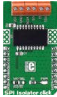
SPI Isolator Click Carries ADuM4154 5kV digital isolator optimized for a serial peripheral interface (SPI). MSRP - $29 00 MIKROE-2583
