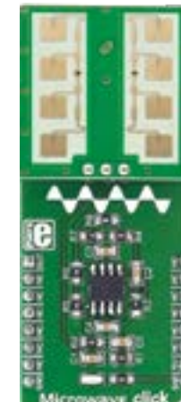
Microwave Click It detects movement, thanks to the PD-V11 a 24GHz microwave motion sensor. MSRP - $25 00 MIKROE-2781
