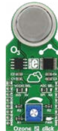
Ozone 2 Click With MQ131 sensor for Ozone [O3]. Detection range 10-1000 ppm of O3.
