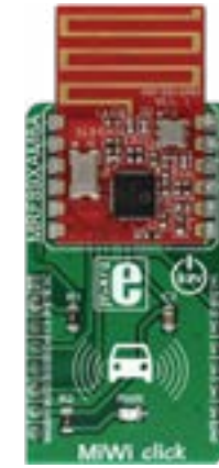
MiWi Click A subgigahertz radio transceiver which offers a reliable FSK or OOK communication solution. MSRP - $17 00 MIKROE-2924
