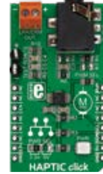
HAPTIC Click With DRV2605 Haptic Driver for ERM and LRA vibration motors. Over 100 haptic effects library. MSRP - $23 00 MIKROE-2025
