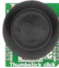
Thumbstick Click A high precision input device with a dual axis, spring return and push-button enabled joystick. MSRP - $20 00 MIKROE-1627
