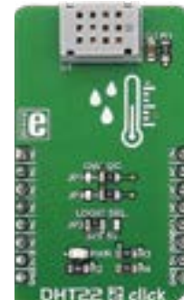
DHT22 2 Click It is used for measuring the environmental temperature and relative humidity. MSRP - $22 00 MIKROE-2818
