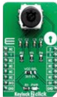
Keylock 2 Click Uses SK13AEG13 switch keylock from the company NKK Switches. MSRP - $28 00 MIKROE-3471
