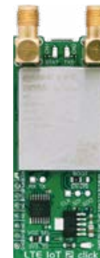
LTE IoT 2 Click Allows connection to the LTE networks, featuring Quectel BG96 LTE module. MSRP - $69 00 MIKROE-3144
