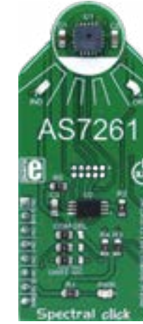
Spectral Click Uses the AS7261, an XYZ chromatic white color sensor + NIR with electronic shutter and smart interface.
