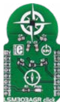
LSM303AGR Click Measures acceleration and magnetic field characteristics. Carries LSM303AGR module.
