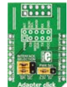
Adapter Click Simplifies connection of the add-on boards with IDC10 headers to mikroBUS™ socket. MSRP - $6 50 MIKROE-1432
