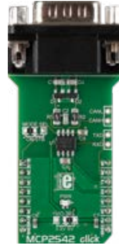
MCP2542 Click Microchip's CAN FD Transceiver with Wake-Up Pattern. Compliant with CAN 2.0 and CAN FD. MSRP - $20 00 MIKROE-2299
