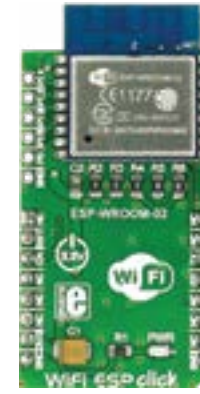
WiFi ESP Click With ESP-WROOM-02 module that integrates ESP8266EX. In AP WiFi and WiFi client mode. MSRP - $15 00 MIKROE-2542
