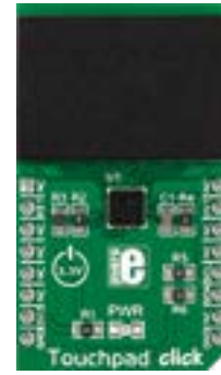
Touchpad Click Capacitive touch input device driven by Microchip's MTCH6102 controller. MSRP - $15 00 MIKROE-1995
