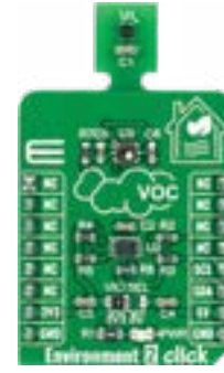
Environment 2 Click The SHT40 and SGP40, a high-accuracy best-in-class SHT relative humidity, and a temp. sensor.
