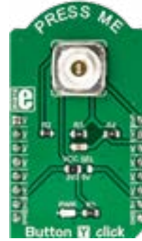
Button Y Click Designed with the high-quality, single-pole, single-throw [SPST] tactile switch labeled as 3006.2111. MSRP - $9 00 MIKROE-3262
