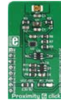
Proximity 6 Click Uses the ADUX1020, a photometric sensor for gesture and proximity detection. MSRP - $29 00 MIKROE-3048
