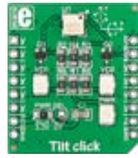
Tilt Click With RPI-1035, a 4-directional optical tilt sensor - left, right, backward, forward movement. MSRP - $12 90 MIKROE-1834
