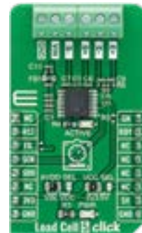
Load Cell 5 Click The AD7780- pin-programmable, low power, 24-bit sigma-delta ADC from Analog Devices.
