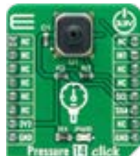
Pressure 14 Click The ABP2LANT060P-G2A3XX, a piezoresistive silicon pressure sensor.
