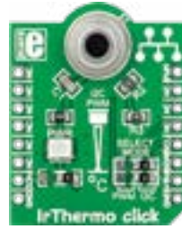
IrThermo Click 5V With MLX90614ESF-AAA IR thermometer module, factory calibrated in wide temperature range.
