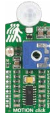
MOTION Click It's a motion detector sensitive only to live bodies with PIR500B, a pyroelectric sensor.
