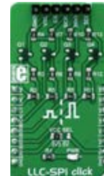
LLC-SPI Click Used as the level converter for logic signals. It is perfectly suited for SPI communication. MSRP - $9 00 MIKROE-3298
