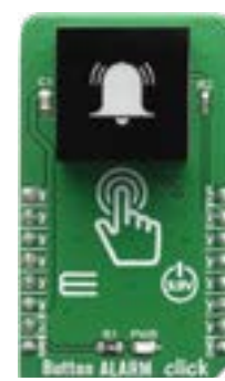
Button ALARM Click With the CTHS15CI-C05ALARM, a capacitive touch sensor display. MSRP - $21 00 MIKROE-3763
