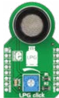
LPG Click With MQ-5 sensor for detecting liquefied petroleum gas leakage. Detection range 200-10000 ppm.
