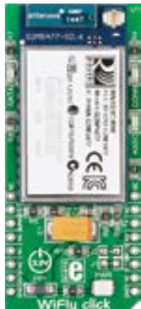
WiFly Click With RN-131 embedded wireless LAN module. Qualified 2.4-GHz IEEE 802.11 b/g transceiver. MSRP - $69 00 MIKROE-1937
