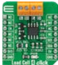
Load Cell 4 Click Features the ZSC31014, a CMOS integrated circuit for highly accurate amplification.
