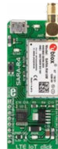
LTE IoT Click Compact quad-band GSM solution, featuring the quad-band SARA-R410M-02B LTE/2G module. MSRP - $79 00 MIKROE-3072
