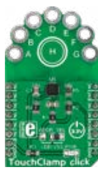
TouchClamp Click With NXP's MPR121 proximity capacitive touch sensor controller. 7 plated holes for clamps. MSRP - $9 00 MIKROE-2294
