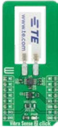
Vibra Sense 2 Click The LDTM-028K a vibration sensor, offering high sensitivity at low frequencies.
