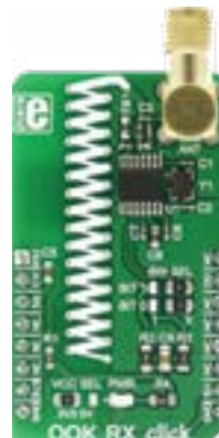
OOK RX Click A wireless receiver that operates at the frequency of 433MHz (sub-GHz). MSRP - $19 00 MIKROE-2902
