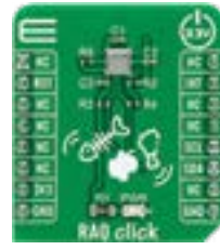
RAQ Click The ZMOD4450, a gas sensor module used to detect typical gases inside refrigeration applications.
