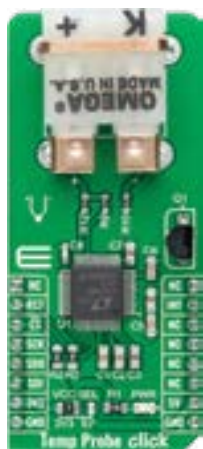
Temp Probe Click The LTC2986, a high accuracy digital temperature measurement system.
