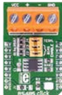
RS485 Click 3.3V Carries SN-65HVD12 half-duplex, RS-485 transceiver from Texas Instruments. MSRP - $18 00 MIKROE-989
