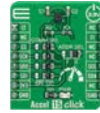
Accel 15 Click The BMA490L, a high-performance 16-bit digital triaxial longevity acceleration sensor.
