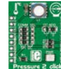
Pressure 2 Click With MS5803, a high resolution MEMS pressure sensor. Range 0-14 bars, resolution up to 0.2 mbars.
