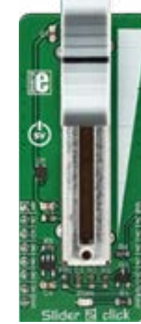
Slider 2 Click Utilizes the PTA3043, a linear, high-grade, 10K potentiometer MSRP - $20 00 MIKROE-3301
