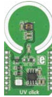
UV Click With ML8511 IC that is sensitive to UVA and UVB rays. Outputs either analog or digital signals. MSRP - $24 00 MIKROE-1677
