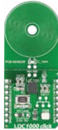
LDC1000 Click With ind-to-digi. converter IC and a detachable inductive sensing.
