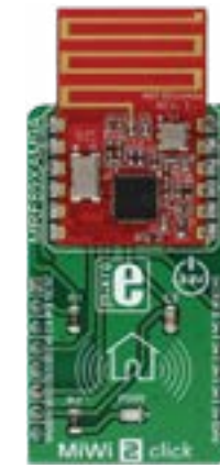
MiWi 2 Click A subgigahertz radio transceiver which offers a reliable FSK or OOK communication solution. MSRP - $17 00 MIKROE-2925
