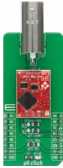
pH Click The pH EZO™, offers the highest level of stability and accuracy from AtlasScientific.
