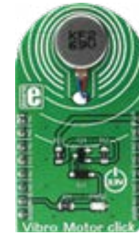
Vibro Motor Click Features a compact size Eccentric Rotating Mass [ERM] motor, labeled as C1026B002F. MSRP - $12 00 MIKROE-2826
