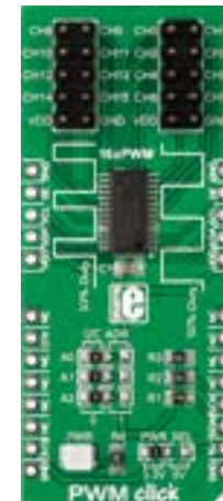
PWM Click For controlling 16 PWM outputs through a single I2C interface. With PCA9685PW IC. MSRP - $14 00 MIKROE-1898
