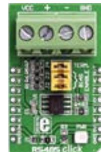
RS485 Click 5V Carries the ADM485 differential line transceiver from Analog Devices. MSRP - $18 00 MIKROE-925
