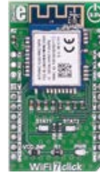
WiFi 7 Click With ATWINC1510-MR210PB IEEE 802.11 b/g/n module, 20MHz solution. MSRP - $29 00 MIKROE-2046
