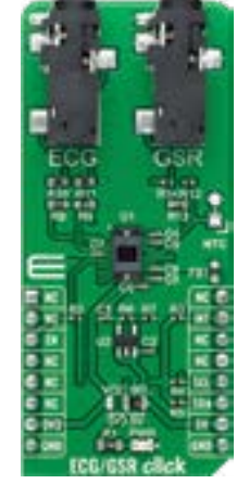
ECG/GSR Click The AS7030B, a vital sign sensor with PPG and Electrocardiogram [ECG] operations.
