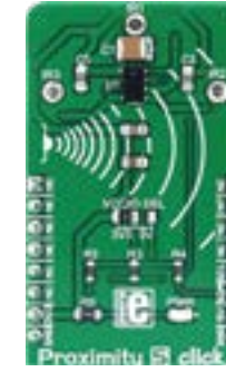
Proximity 5 Click Features the VCN-L4035X01 J, a fully integrated proximity and ambient light sensor. MSRP - $15 00 MIKROE-2984
