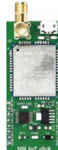
NB IoT Click Allows LTE Cat NB1 connectivity by utilizing Quectel BC95-G MSRP - $52 00 MIKROE-3294
