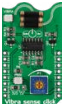
Vibra sense Click A micro shock vibration sensor with a digital output. For anti-tampering, anti-theft devices. MSRP - $18 00 MIKROE-1927
