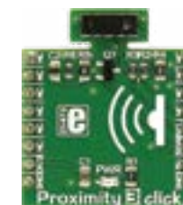
Proximity 3 Click Intelligent proximity and light sensing device - high sensitivity long distance PS and ALS. MSRP - $17 00 MIKROE-2801
