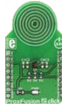
ProxFusion® 2 Click The IQS621, a multi-functional sensor with the ambient light [ALS] from Azoteq. MSRP - $9 00 MIKROE-3205
