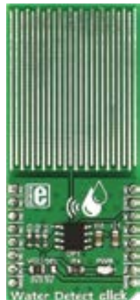
Water Detect Click For detecting water and other electroconductive liquids. Carries Microchip's MCP606. MSRP - $9 00 MIKROE-2786
