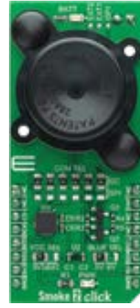
Smoke 2 Click The ADPD188BI module for smoke detection with optical dual-wave-length technology.
