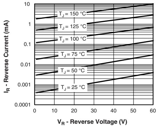
Fig. 2 - Typical Peak Reverse Current vs. Reverse Voltage
