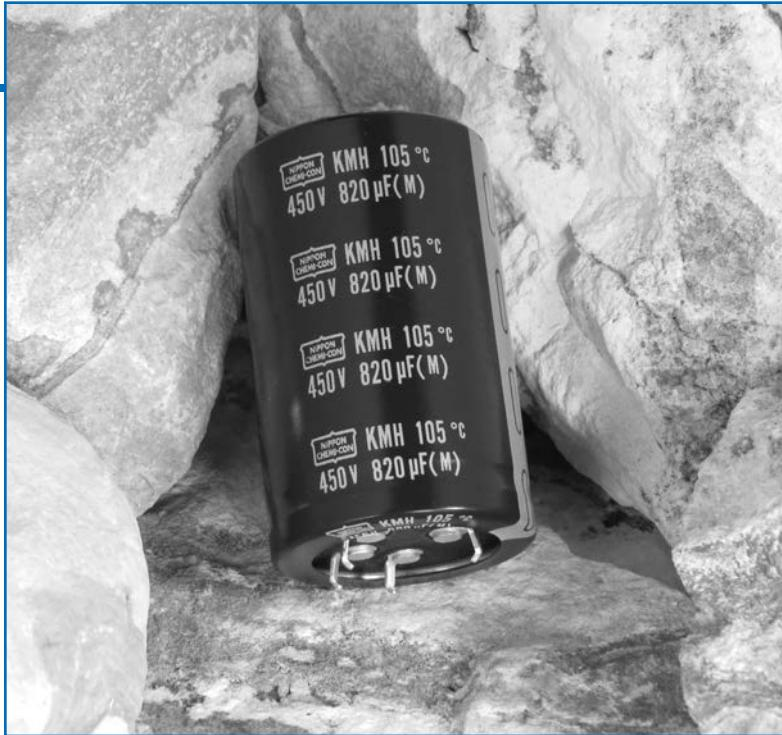
The KMH series capacitors are the standard +105°C high temperature, large capacitance snap-in capacitors that offer a wide voltage range of 6.3 to 450VDC. The endurance for the KMH series is 2,000 hours at +105°C with the rated ripple current applied. With very high CV values and high ripple current capabilities these capacitors are ideal for use in power supply filter circuits.
