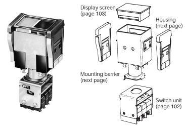
Mounting barriers attach to either the long or short sides of the housing. They have spring clips which grip the panel. Mounting barriers also separate display screens to protect against inadvertent operation. Multiple units can be attached together in a strip and snapped into a panel slot; or they can be mounted individually.
