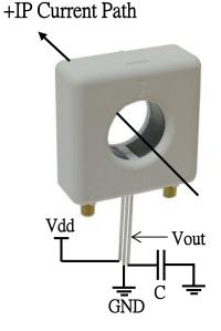
Capacitor  $C(0.01 \mu F \sim 0.1 \mu F)$  is recommend to be connected between Vout and GND to reduce output noise.
