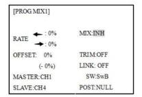
AT9S Pro contains four separate linear programmable mixes. (Note that mixer #5-8's mixing RATE are set with a 5-point curve. HELI has mixer #5-6's mixing. See CURVE MIXES
