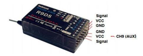
(2) SBUS&PWM dual signal output working mode: blue/purple LED indicates SBUS&PWM signal output at the same time with 10 channels totally. CH9 outputs SBUS signal while the original CH1 outputs CH3 PWM signal and original CH2 to CH6 output CH6 to CH10 PWM signal at the same time.
