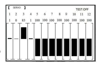
• Servo cycle function to help locate servo problems prior to in-flight failures. (Channels 1-8)
