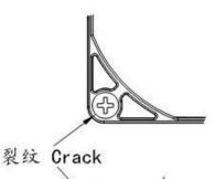
\* 考虑到车架裂纹,禁止使用锥度螺钉。 Taper screw is prohibited for frame crack consideration.
