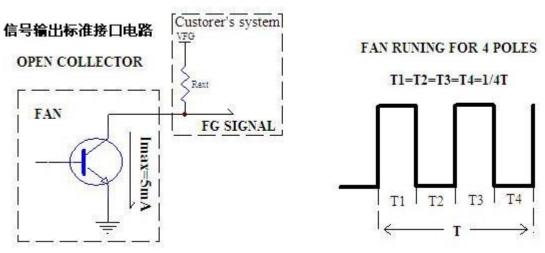
VFG= 5-24 Vmax Rext (min) = VFG/Imax Imax=5mA Vce=0.5Vmax 13.3. N=RPM T=60/N(SEC) T1=T2=T3=T4=1/4T
