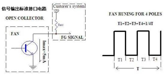
VFG= 5-24 Vmax Rext (min) =VFG/Imax Imax=5mA Vce=0.5Vmax
