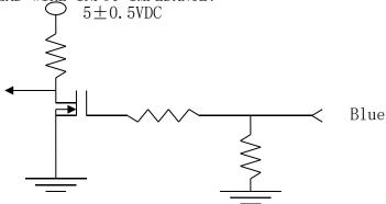
1. THE FAN SPEED WILL DEFAULT TO MAXIMUM WHEN THE SPEED CONTROL INPUT IS LEFT UNCON
