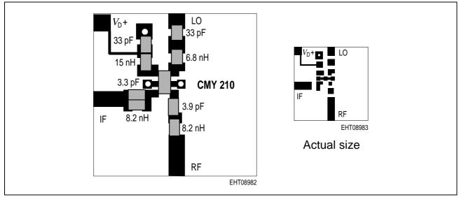
Figure 2 PCB-Layout for 800 MHz Test and Application Circuit
