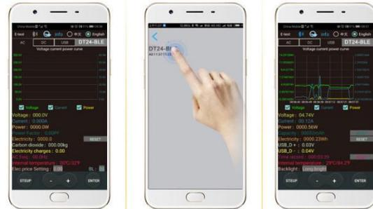
**1** When the USB tester is powered on, the Bluetooth indicator is flashing, turn on the E-test App software icon, and allow Bluetooth to turn on.
