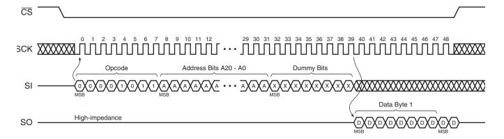
Figure 26-2. Continuous Array Read Timing (Opcode 0Bh)
