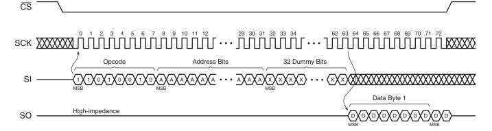
Figure 26-4. Main Memory Page Read Timing (Opcode D2h)
