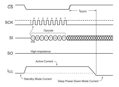
Figure 11-1. Deep Power-Down Timing
