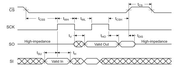
Figure 23-1. Waveform 1 = SPI Mode 0 Compatible
