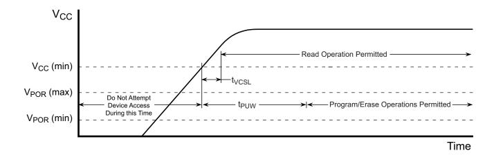
Figure 17-1. Power-Up Timing
