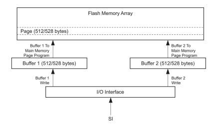
Figure 24-1. Block Diagram
