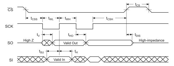
Figure 23-2. Waveform 2 = SPI Mode 3 Compatible
