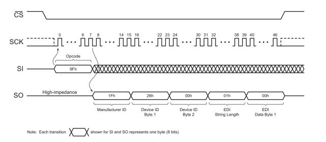
Figure 13-1. Read Manufacturer and Device ID Timing
