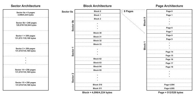
Figure 4-1. Memory Architecture Diagram
