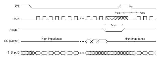
Figure 26-12. Reset Timing
