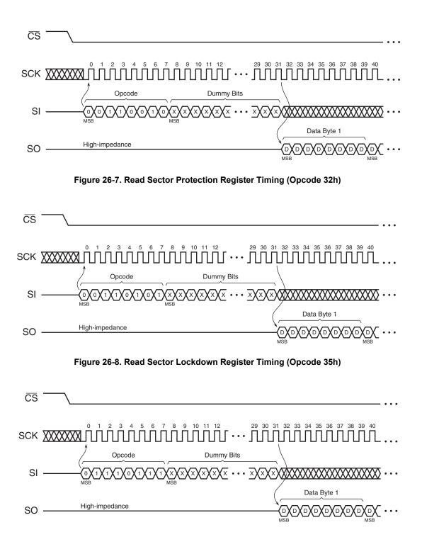
Figure 26-9. Read Security Register Timing (Opcode 77h)
