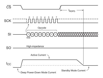
Figure 11-2. Resume from Deep Power-Down Timing
