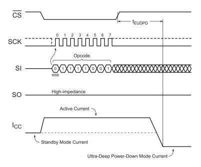
Figure 11-3. Ultra-Deep Power-Down Timing
