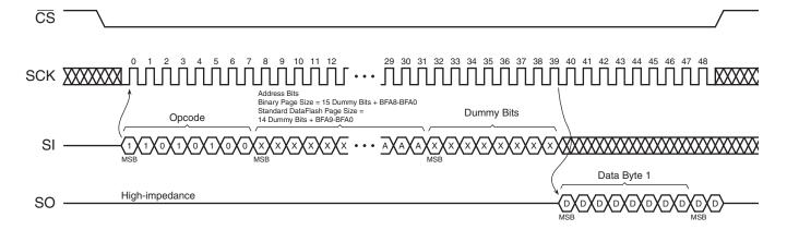
Figure 26-5. Buffer Read Timing (Opcode D4h or D6h)
