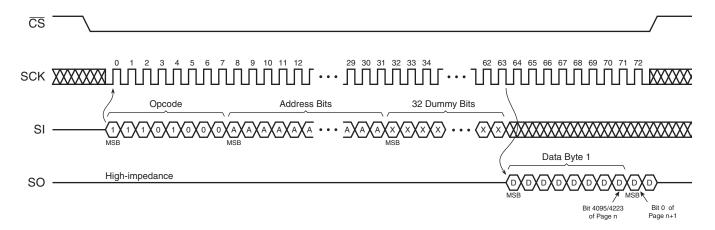
Figure 26-1. Continuous Array Read Timing (Legacy Opcode E8h)
