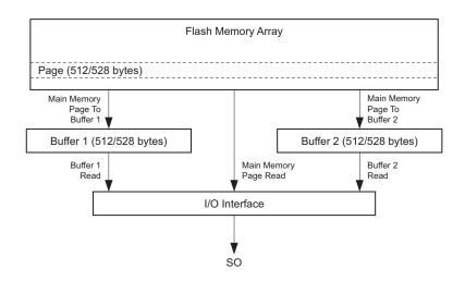
Figure 25-1. Block Diagram
