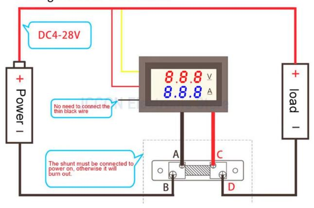
4. Wiring diagram of independent power supply for Tange 50A or 100A meter
