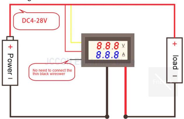
2.Wiring diagram of independent power supply for Tange 1A or 10A meter
