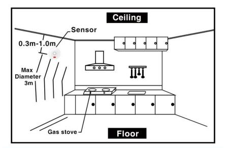
1. First of all, it is necessary to determine whether the detected gas is heavier or lighter than air. Gases heavier than air: liquefied petroleum gas, etc.; gases lighter than air: natural gas, artificial gas, biogas, etc.
