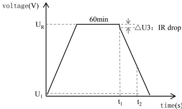
容量计算方式 Capacitance calculation :  $C = I \times \frac{t_2 - t_1}{U_1 - U_2}$
