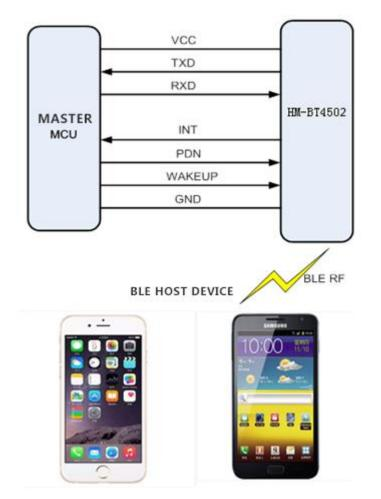
Figure 1. Application Schematic of the Pass-through Module
