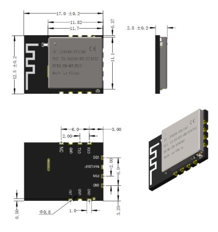
Fig4. HM-BT4502 Module Size Diagram
