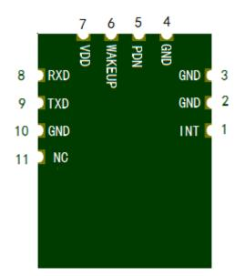
Fig. 3. Module Pins Distribution Diagram (Bottom View)
