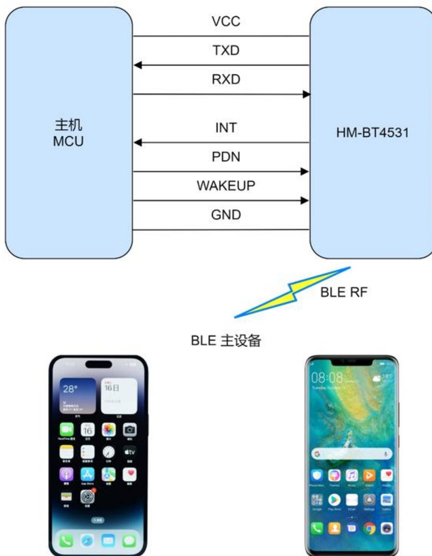
Figure 1 Application Diagram of Transparent Transmission Module
