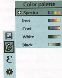
As shown in the figure, press "⏏/MENU" key to enter the main menu and select "🎨" (color palette) option and press "▶" key to enter the color palette list. Press "▲" and "▼" keys in navigation to select the color palette. Then press "SELECT/ENTER" key to select the color palette. Press "◀" to return. Press "⏏/MENU" key to exit from the menu.
