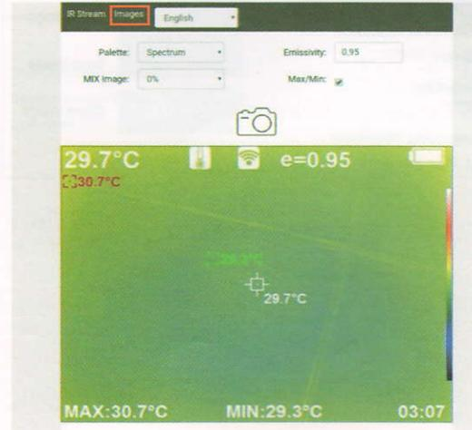
Click "Image" in the mobile device to enter the image view, press the image to download the image, long press the image to save to the mobile device, click "Infrared Video Stream" to return to the video stream webpage, as shown below.
