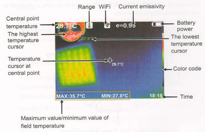
Range: The range of temperature measurements.
