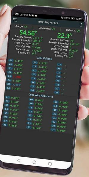
Download the specified Bluetooth application and activate the BMS. Open the Bluetooth application and find the relevant serial number, then you can check all the data.
