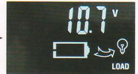
8: Discharge cut-off voltage setting
