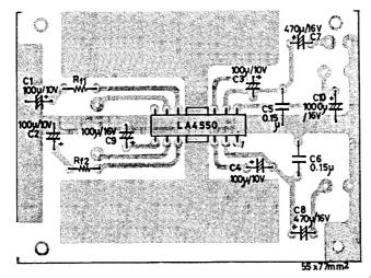
Sample Printed Circuit Pattern (Gu-foiled area) for Stereo Use
