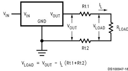
**FIGURE 3. Typical Application using Fixed Output Regulator**
