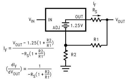
$$I_F = \frac{V_{OUT} - 1.25 \left(1 + \frac{R2}{R1}\right)}{-R_S \left(1 + \frac{R2}{R1}\right)}$$
