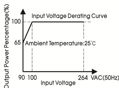
Note: 1. With an input voltage between 90-100VAC the output power must be derated as per the temperature derating curves;
