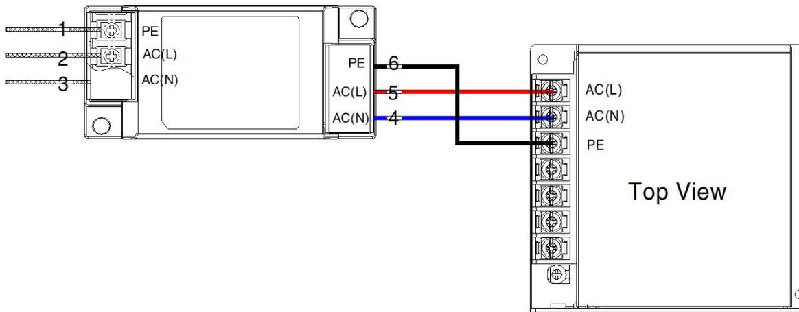
Fig. 1: EMC application circuit with higher requirement
