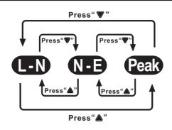
Voltage (V<sub>d</sub>): real time display of cable connection status and display the voltage drop of current load and measurement results of phase voltage drop TRMS. This test item includes 3 submenus, namely load with 5A, 8A and 10A. Press Up " ▲" or Down " ▼" selection key on the sub test item to enter the relevant test item.
