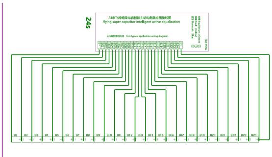
For the battery pack with 24 cells,
