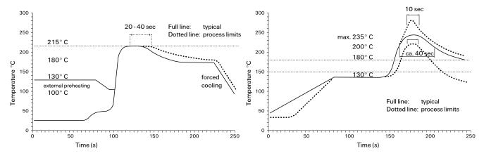
Vapor Phase Soldering: Temperature/Time Profile (Lead Temperature)
