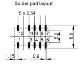
Note: Solder pad for pin 6 and 7 only for latching with 2 coils
