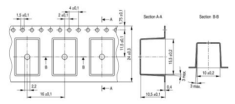
Tape and reel for SMT version with short terminals - 500 relays per reel, 2500 relays per box
