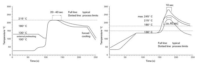
Vapor Phase Soldering: Temperature/Time Profile (Lead Temperature)
