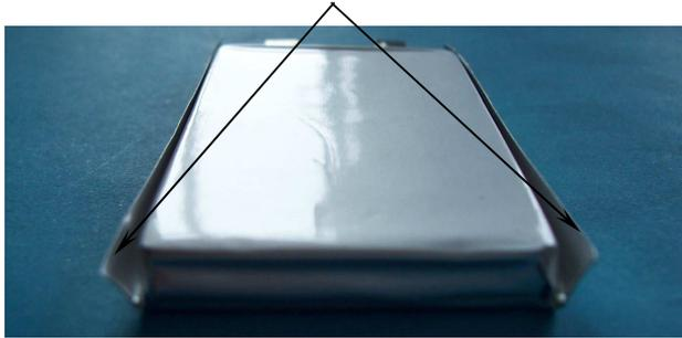
Fig.2. Single folding edge schematic of PL cells
