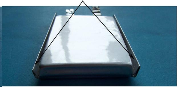
Fig.3. Reverse folding edge schematic of PL cells
