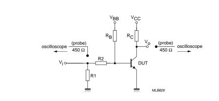
$V_i$  = 0.5 to 4.2 V; T = 500  $\mu s;$   $t_p$  = 10  $\mu s;$   $t_r$  =  $t_f \leq 3$  ns.
