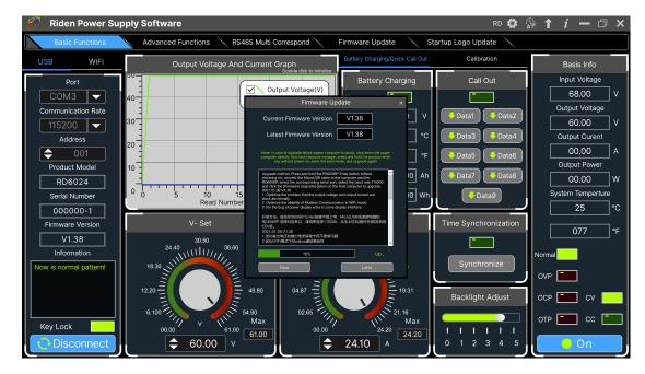
During the firmware upgrade process, the interface is displayed as follows:
