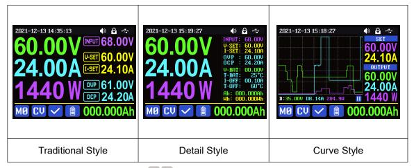
At main page you can press button to change the display style between Traditional Style, Detail Style and Curve Style, the display style will not be saved automatically, you need to set default boot display at section 1.4.2.6 Main Page Style Setting.
