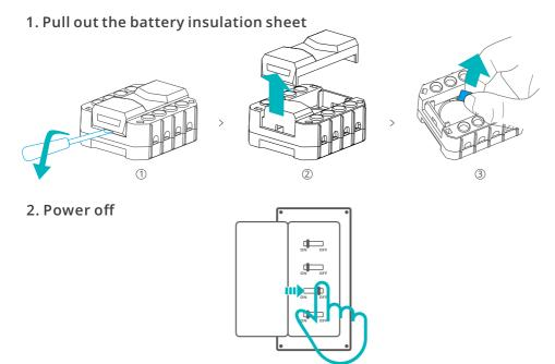
Please install and maintain the device by a professional electrician. To avoid electric shock hazard, do not operate any connection or contact the terminal connector while the device is powered on!
