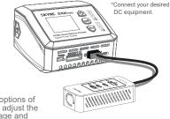
Select the options of DC Power: adjust the output voltage and current.
