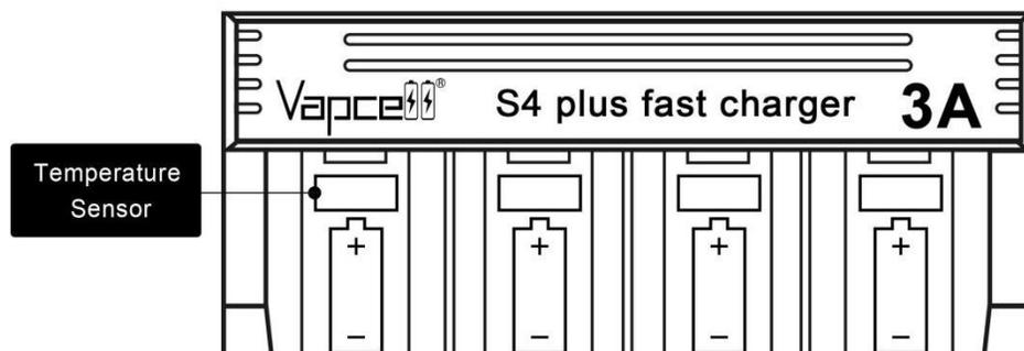
1. Temperature is higher than 65 °C. If the charging current is higher than 1500 mA (excluding 1500 mA), it will be reduced to 2 level, for example your current charge current is 3000mA, it will be automatically charged at 2000mA.
