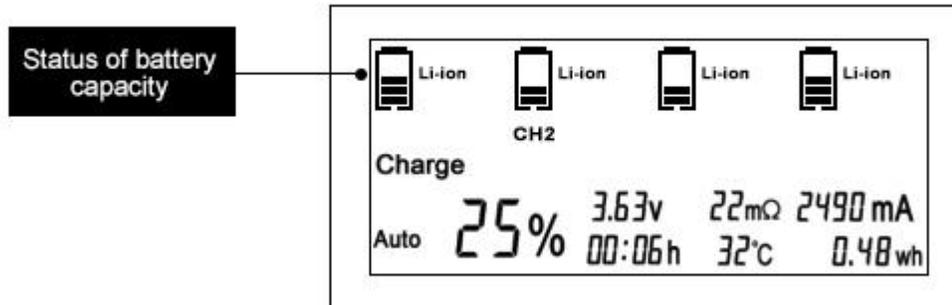
2.7 If multiple batteries are placed in the charger at the same time, we press the DISPLAY button several times to display the battery data of each slot in turn. Each slot is independent of each other, there are slots to charge, there are slots to discharge, there are slots to repair the process, without interference with each other. If CH1 is displayed, it will be the data of the first slot battery.
