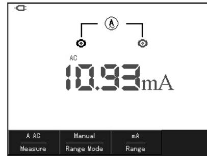
Picture 5-11 Measurement of AC Current lower than 400mA
