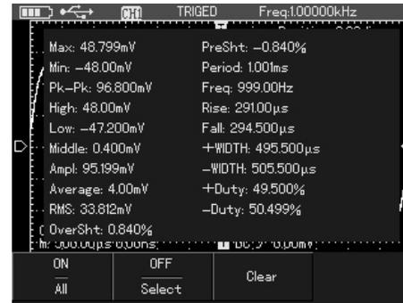
Picture 6-16 All Parameters Measurement
