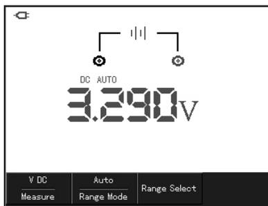
Picture 5-5 DC Voltage Measurement
