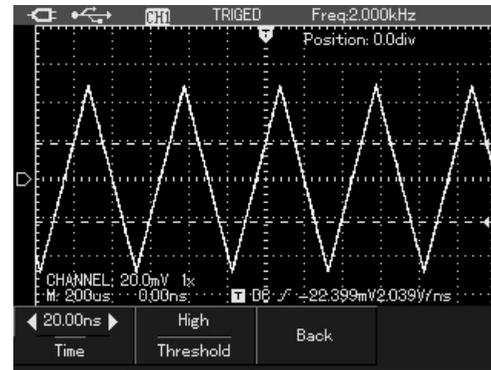
Picture 6-13 the Second Page of Trigger-Slope Trigger
