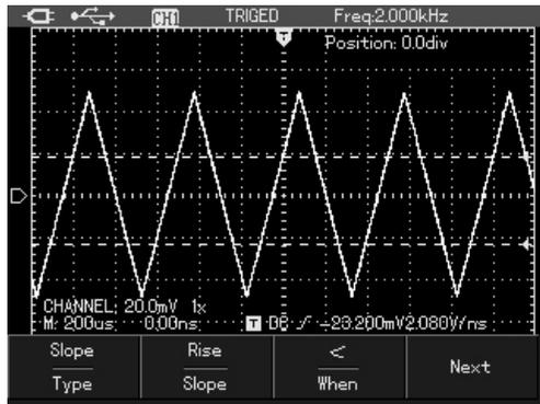
Picture 6-12 the First Page of Trigger-Slope Trigger
