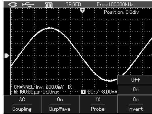
Picture 4-23 opposite phase display of waveform
