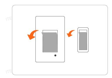
① Tear off the protective film of the 3M adhesive.
