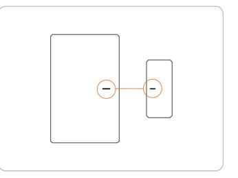
② Try to align the mark line on the magnet with that on the transmitter during installation.
