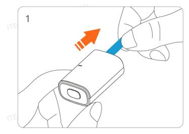
Take out the battery insulation sheet to power on the device
