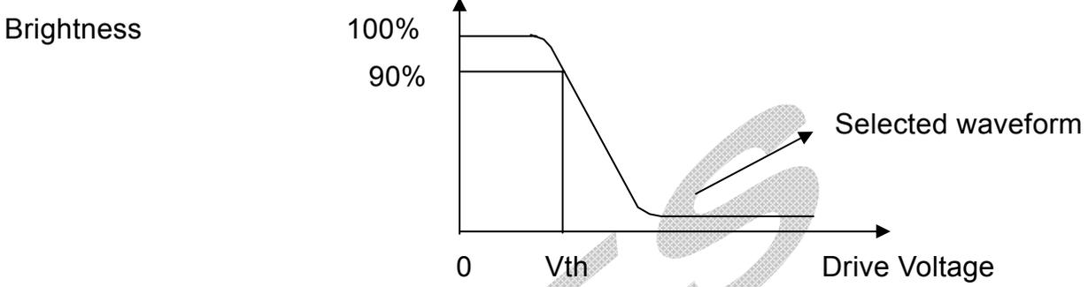
Vth: the voltage (Vop) which the brightness of segment indicates 10%,of saturated value on conditions.
