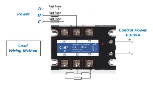
Y Load Wiring Method
