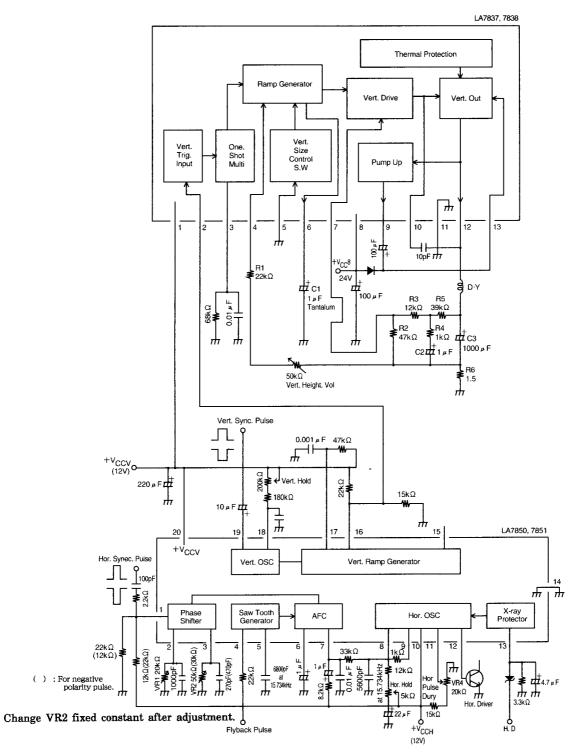
Sample Application Circuit : 14" Color Monitor/ $f_V$ =60Hz,  $f_H$ =15.734kHz
