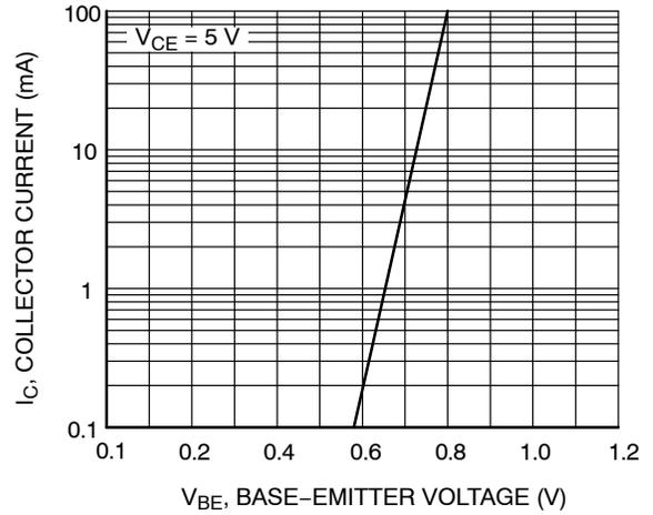
Figure 2. Transfer Characteristics
