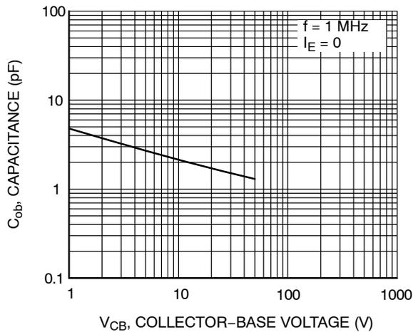
Figure 5. Output Capacitance
