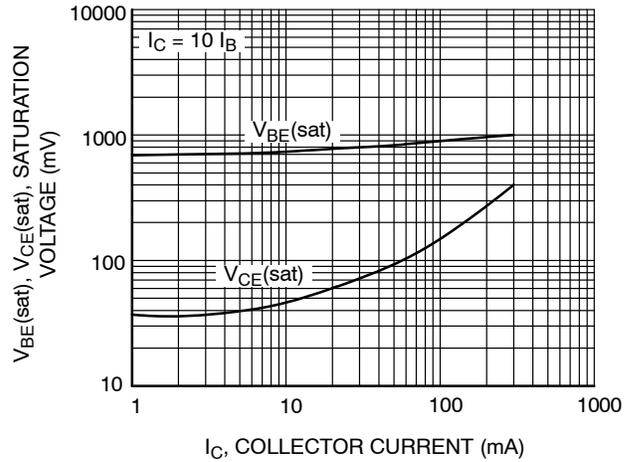
Figure 4. Base-Emitter Saturation Voltage and Collector-Emitter Saturation Voltage
