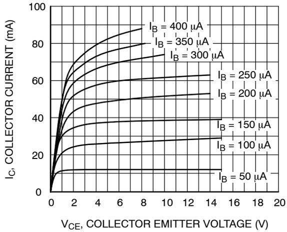
Figure 1. Static Characteristic
