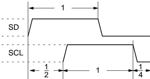
Fig. 2-20: Start condition I<sup>2</sup>C bus
