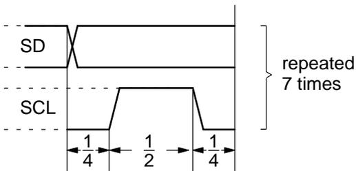
Fig. 2-21: Single bit on I<sup>2</sup>C bus
