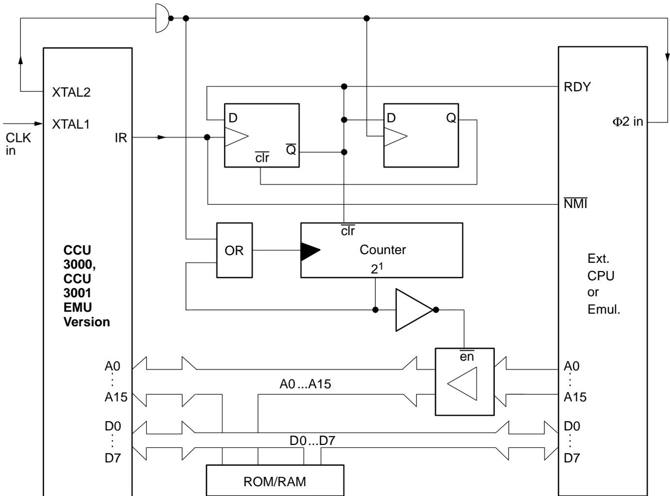
Fig. 2-12: Using an external CPU
