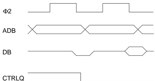
**Fig. 2-10:** Static control signals interrupt
