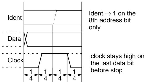
Fig. 2-24: Single bit on IM bus
