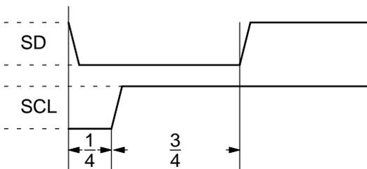
Fig. 2-22: Stop condition I<sup>2</sup>C bus
