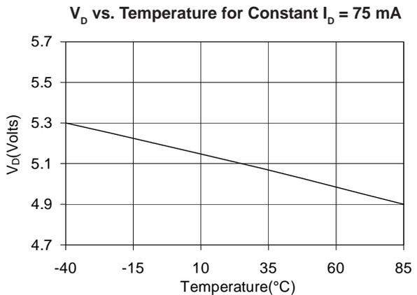
\* Note: In the applications circuit on page 4,  $R_{BIAS}$  compensates for voltage and current variation over temperature.
