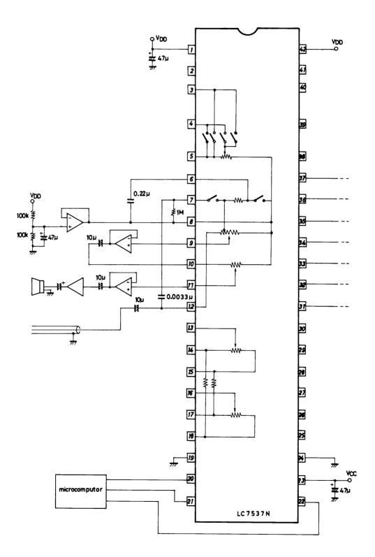
Unit (resistance:  $\Omega$ , capacitance: F)
