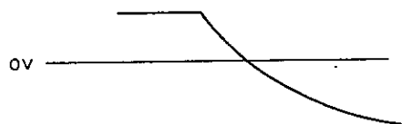
Fig. 1 Voltage of pin 7 as FS1 changes from 0 to 1
