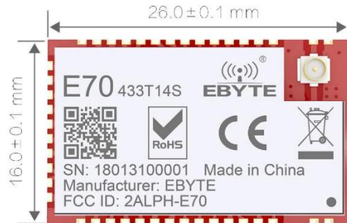
The module features FEC (Forward Error Correction) algorithm, which ensure its high coding efficiency & good correction performance. In the case of sudden interference, it can correct the interfered data packets proactively, so that the reliability & transmission range are improved correspondingly. But without FEC, those data packets can only be dropped.
