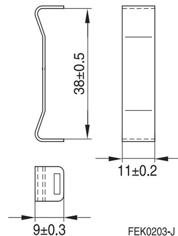
**Coil former** (magnetic axis vertical)
