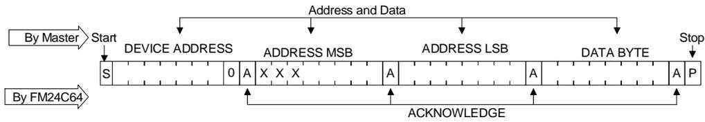
Figure 5. Byte Write
