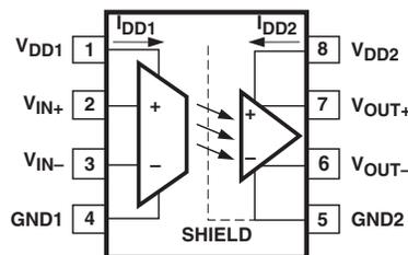
A 0.1 μF bypass capacitor must be connected between pins 1 and 4 and between pins 5 and 8.
