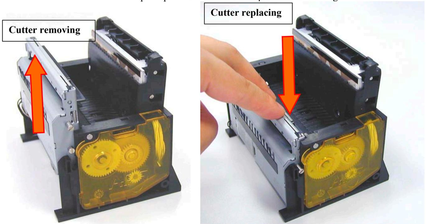
To replace the cutter in position, align the metallic pins with the lateral guide and push downwards until the cutter is in position.
