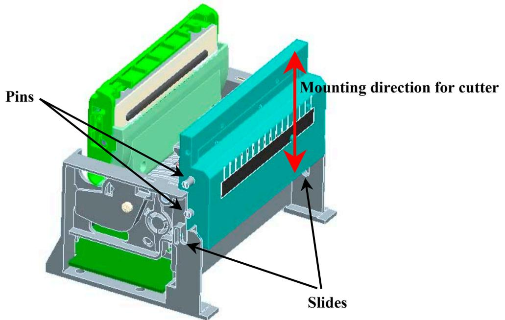
**Fig. 1 – cutter installation**
