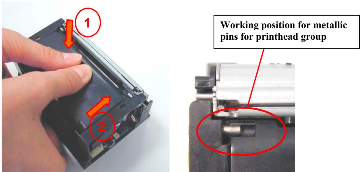
To open the thermal head push slightly downwards with 2 fingers and, keeping pushed downwards, pull backwards. The group can be rotated up to 90°.
