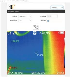
Click "Image" in the mobile device to enter the image view, press the image to download the image, long press the image to save to the mobile device, click "Infrared Video Stream" to return to the video stream webpage, as shown below.
