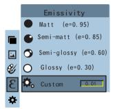
As shown in the figure, press "  $\circlearrowleft$  / MENU" key to enter the main menu and select "  $\circlearrowright$  " (emissivity) option and press "  $\blacktriangleright$  " key to enter the emissivity list.
