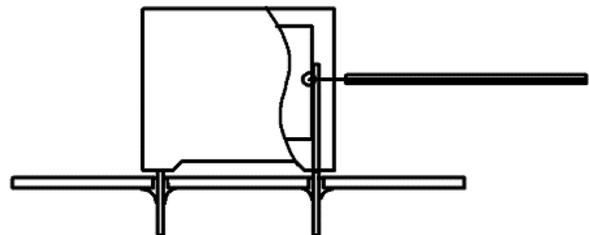
*Temperature monitored inside the capacitor.*
